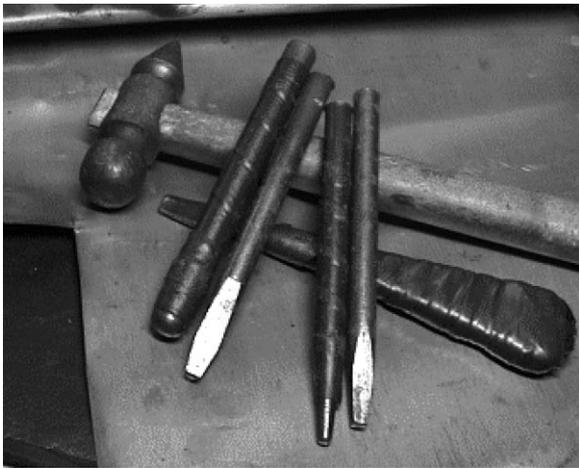
Fig. 9. Tools used for chasing on metal.
